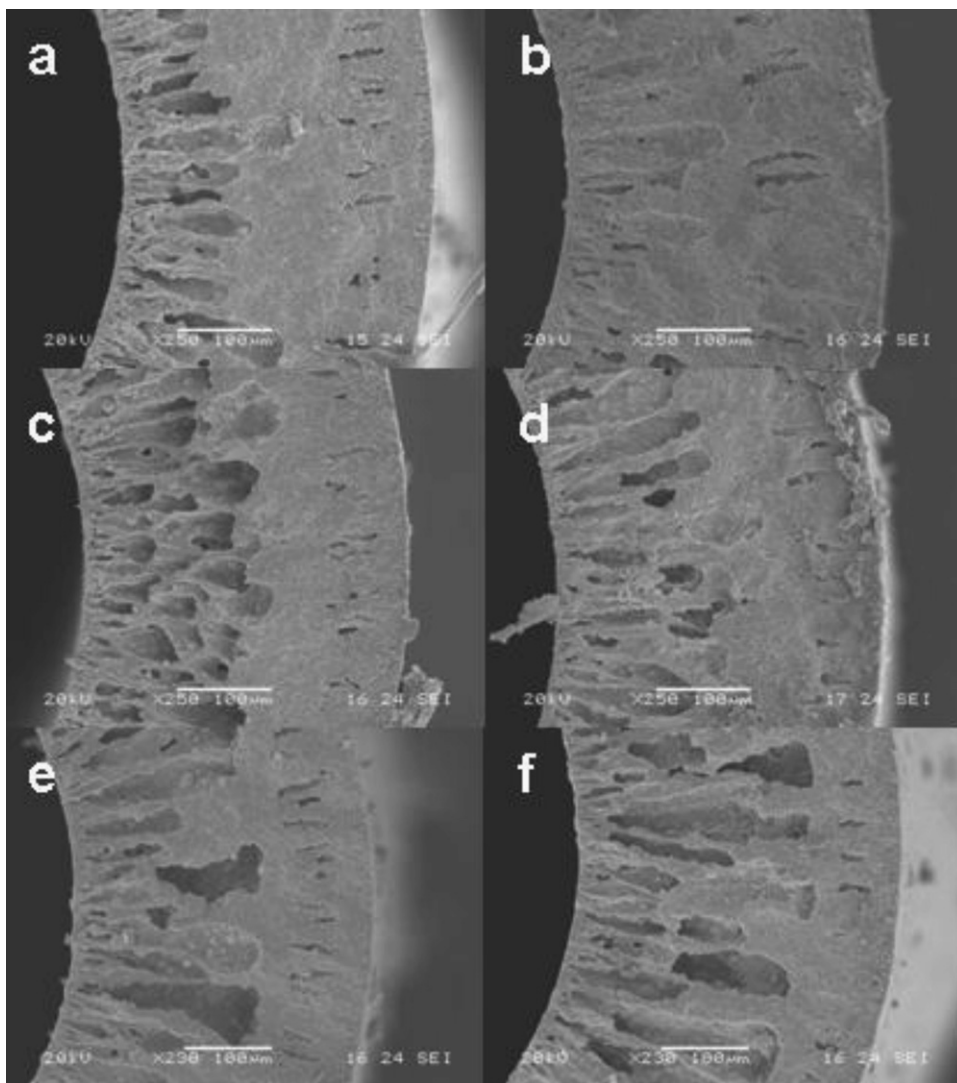
Fig. 13. Cross-sectional SEM images of fibres prepared with air-gaps between 3 and 13 cm and with an internal coagulant flow rate of 7 mL/min calcined at 1450 °C: (a) 3 cm, (b) 5 cm, (c) 7 cm, (d) 9 cm, (e) 11 cm and (f) 13 cm.
